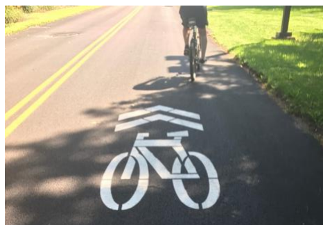
A lane shared by vehicles and bikes, indicated by a sharrow (Photo: VTC)
